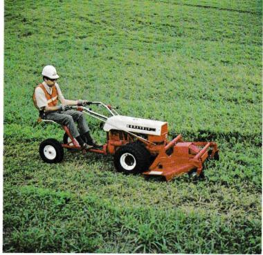
Gravely 10 hp Convertible Tractor with 40 inch Rotary Mower,Sulky, Dual Wheels
