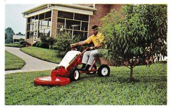
Gravely 7.6 hp Convertible Tractor with 30 inch Rotary Mower, Riding Sulky, Optional Chain Guard
