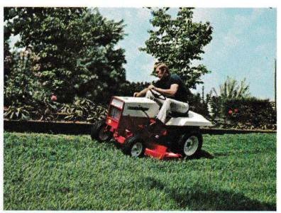
Gravely 432, 14 hp Riding Tractor with 50 inch Rotary Mower
