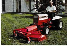
Mow the grass ahead of the tractor — 50 inch Frontmount Rotary Mower
