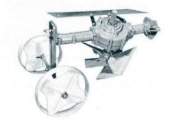
SPECIFICATIONS: 15578E1 Rotary Plow Drive: splined steel shafts, bevel gears, completely enclosed. Plow: four blades, high carbon steel, forged cutting edges.
