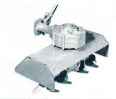
SPECIFICATIONS: 15579E1 Rotary Cultivator Drive: splined steel shafts, gears, fully enclosed. Tines: 16, high carbon steel, forged. Cutting Depth: 3 inches. Width: 26 inches. Height: 19 inches. Length: 10 inches. Attaches to: Rotary Plow Drive Assembly.
