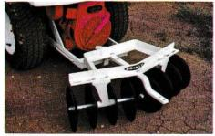
**MODEL DD-500 LIFT TYPE DISC HARROW**
