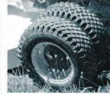
DUAL WHEELS Doubles tire surface for better traction-adds weight, lowers center of gravity. Recommended for slopes, rough terrain, in snow.
